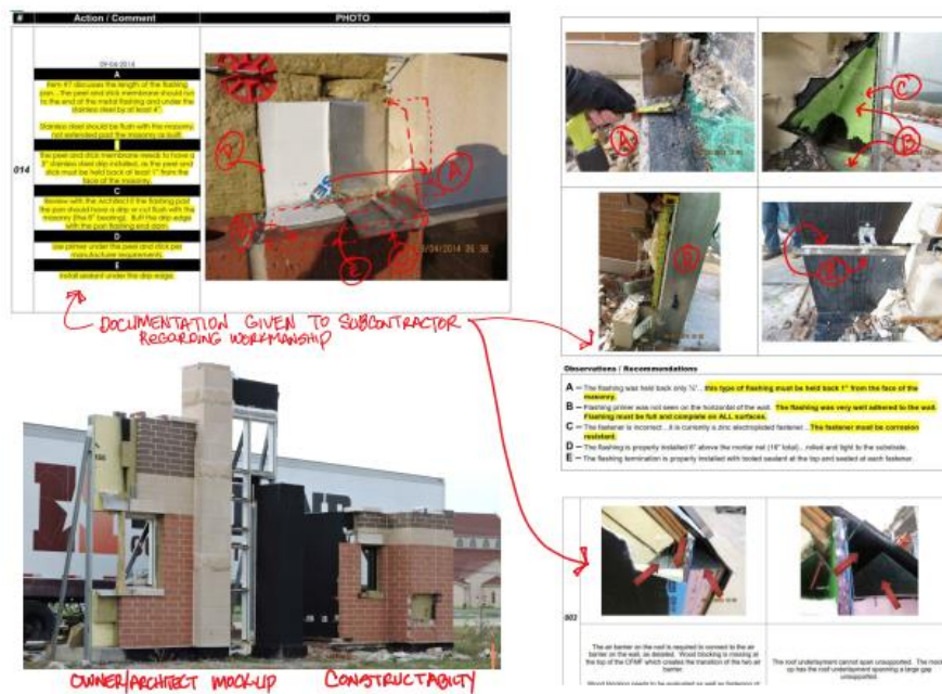
Figure 4. Masonry constructability mock-up review report
